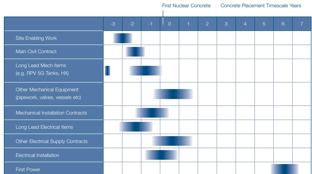
The current view is that EDF Energy first nuclear concrete date for Hinkley Unit 1 will be 2013. For Horizon Nuclear Power the equivalent date for the first unit at Wylfa is likely to be late 2013. There is less certainty regarding first nuclear concrete for NuGeneration Ltd at Sellafield but 2015 is possible.
