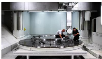
Inside one of the Nuclear AMRC's large-scale state-of-the-art machining cells, a Dörries Contumat vertical turning/milling lathe.
