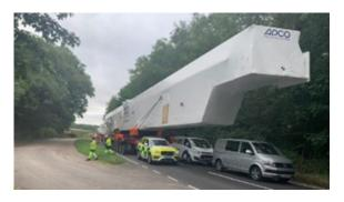
Meanwhile, the last major components for Unit 1's polar crane have arrived at HPC. The two beams will eventually carry the large gantry polar crane as it swivels around the dome of the reactor building and manoeuvres heavy components into place during construction, maintenance work and refuelling.
