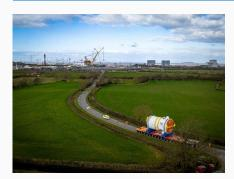
The first new nuclear reactor for a British power station for more than 30 years has arrived in Somerset. At just 13-metres long and weighing 500-tonnes, the "reactor pressure vessel" will create the heat needed to make steam for the world's largest turbines.
